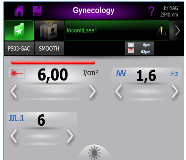
Figure 6: Application screen for IncontiLase showing burst of six SMOOTH pulses per each location
