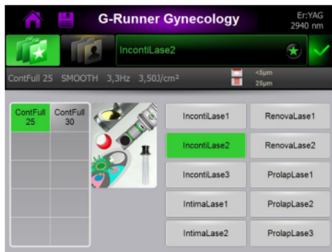
Figure 17: Applications library screen for the second step of the G-runner IncontiLase Treatment protocol with GClear25 speculum. The image at the centre of the screen shows the correct configuration of the components needed for this step
